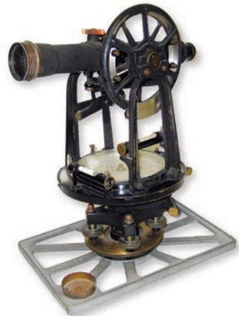
This 1919 'Engineers Transit' model 5060A made by Keuffel & Esser was used by Dickson at the beginning of his career when he worked for the South Carolina Department of Transportation. This item continued to be operated by firm surveyors for several decades thereafter.
